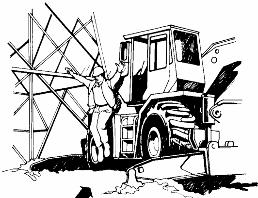
RIGHT (BUT STILL DANGEROUS) The operator should never leave the machine unless absolutely necessary.
