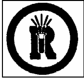
Dangerously Reactive Material
